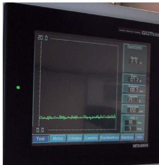
Dynamic stress control test of the roller and its bearing performance.
