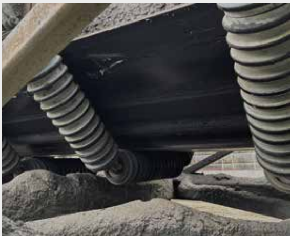
Heavy-duty garland Cap. 18,800 t/h Speed 7.5 m/s BW 2,000 mm
